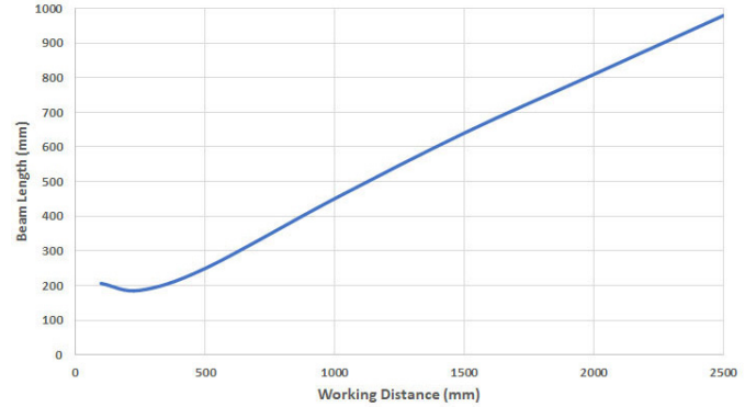
Lens Position 3: Beam Length (80% max) vs. Working Distance
